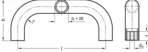
$\begin{array}{ll} d1 &= 28 \\ d2 &= M10 \\ h &= 78 \\ I &= 400 \\ r &= 32 \\ t \mbox{ min} = 15 \end{array}$
